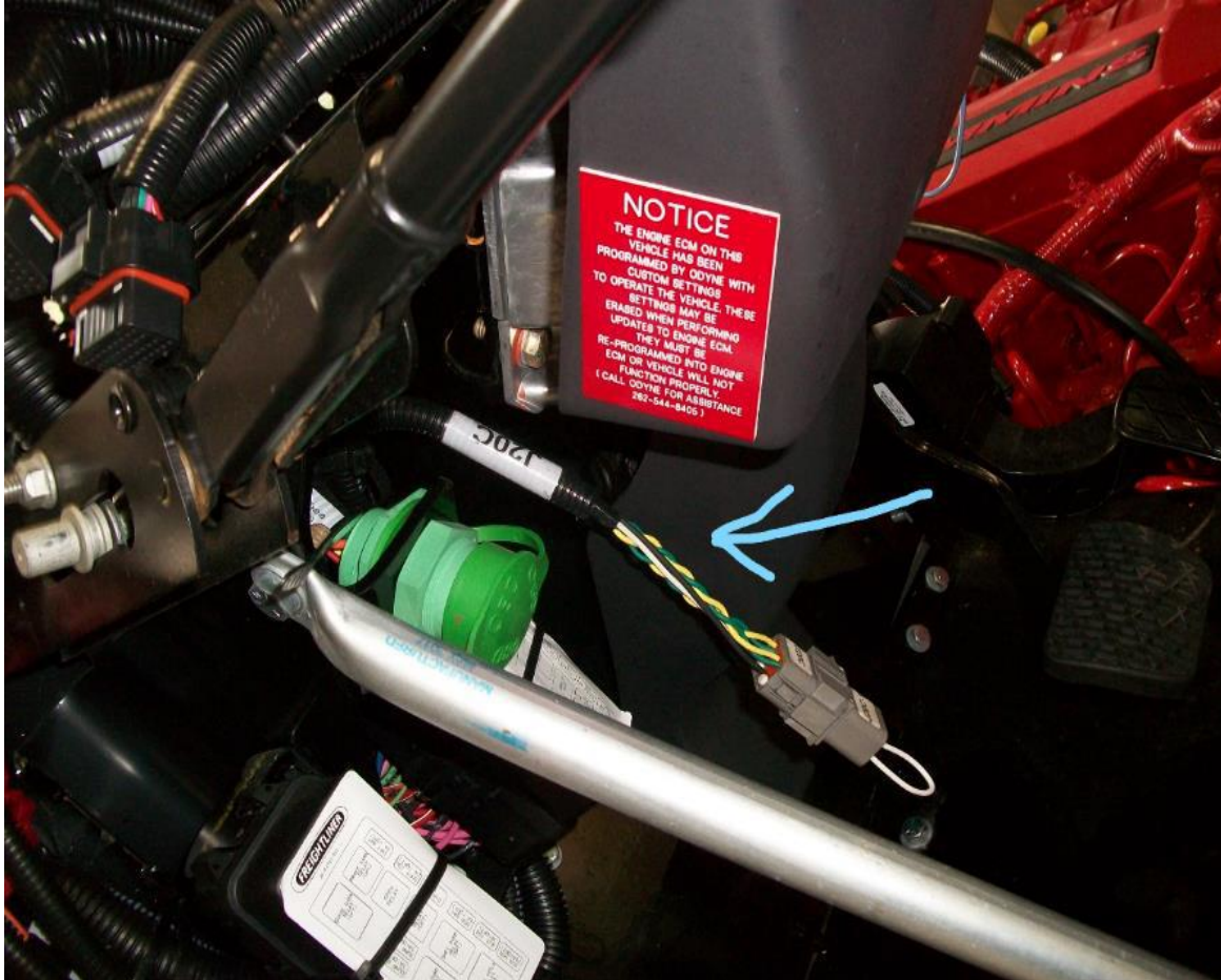
Pic B: On a G2V3 truck and newer there is a female plug for our data connector J20C (shown below)
