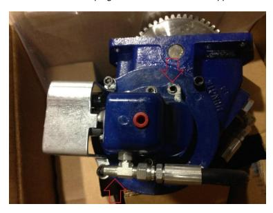
2. Remove the two Allen plugs, exposing the drag brake springs.
